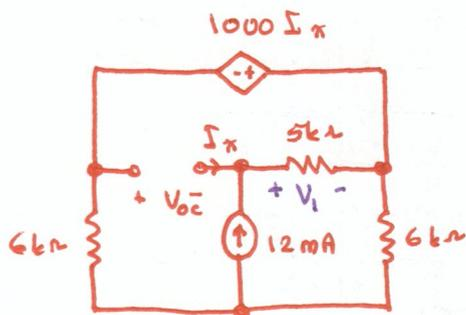
$$I_x = 0 \Rightarrow V_{\pi} = (5\text{k}\Omega)(12\text{mA}) = 60\text{V}$$
