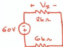
$$V_x = - \frac{2\text{k}\Omega}{2\text{k}\Omega + 6\text{k}\Omega} (60\text{V}) = -15\text{V}$$
